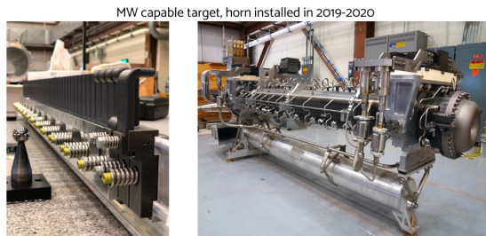
MW capable target, horn installed in 2019-2020
