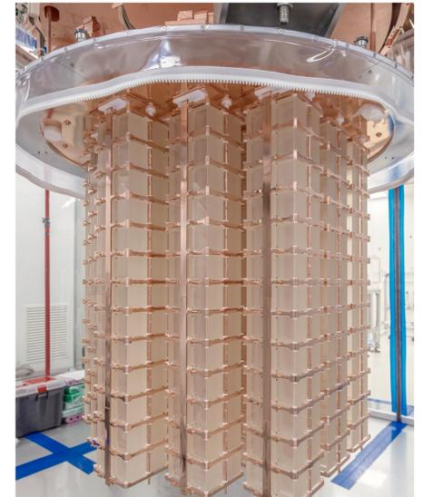
CUORE [1], the largest presently operating cryogenic calorimetric  $0\nu\beta\beta$  search with 988  $\text{TeO}_2$  detectors
