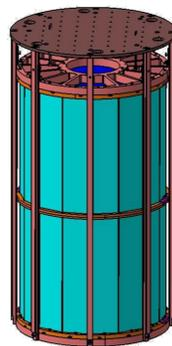
Active high density/radiopurity shield at 10 mK
