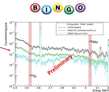
BINGO Geant4 simulation in CUORE shielding (copper surface) -  $\text{O}(x 10)$  improvement from surface contaminations possible
