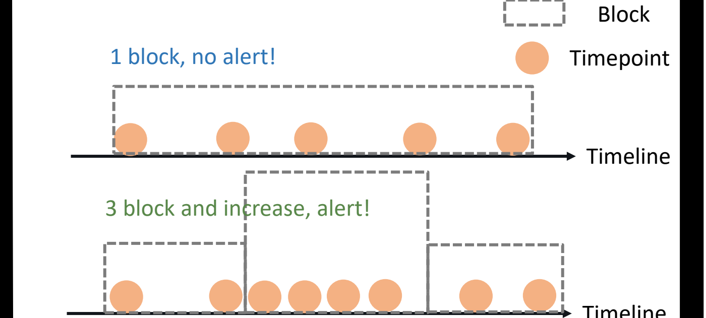
Figure 8: BBA will generate more than one block when time series are clustered.
