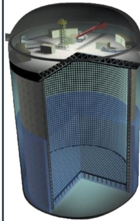
Super-K: 22.5 kton water Cherenkov detector located in Kamioka mine in Japan. In operation since April 1996.
