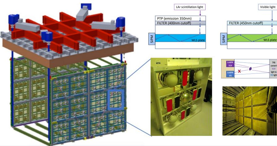
**Active elements:** on the PD-BOX, behind the anode.
