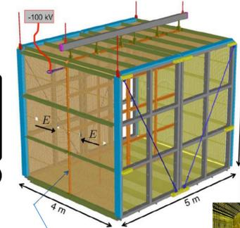
**Cathode Plane at -100 kV** divides the detector into 2 drift volumes. Drift distance is 2 m, drift time is 1.28ms
