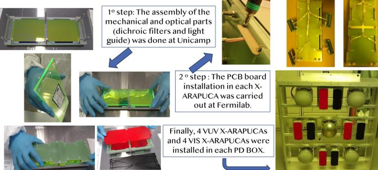
1° step: The assembly of the mechanical and optical parts (dichroic filters and light guide) was done at Unicamp
