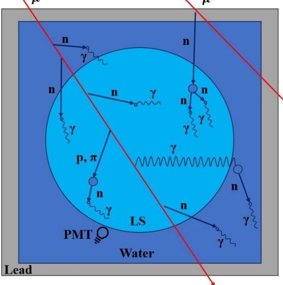
Due to the finite volume of detector, the spill of neutron and gamma is complex for the measurement of yield. An overall detector simulation is conducted to evaluate these effects.
