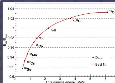
Calibration source energies used to measure non-linearity [5]
