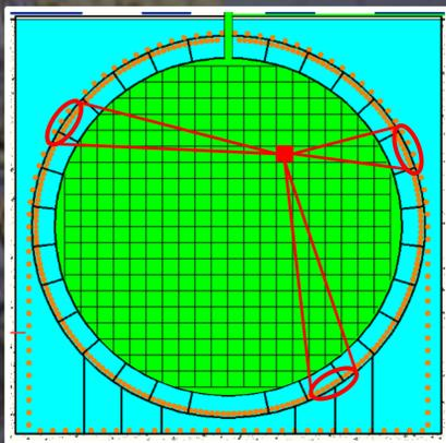
Sketch of the division of the detector into "voxels". The expected PMT charge collection can be calculated for each.
