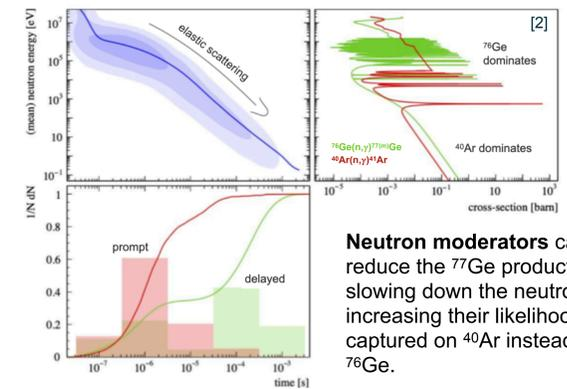
**Neutron moderators** can reduce the  $^{77}\text{Ge}$  production by slowing down the neutrons and increasing their likelihood to be captured on  $^{40}\text{Ar}$  instead of  $^{76}\text{Ge}$ .
