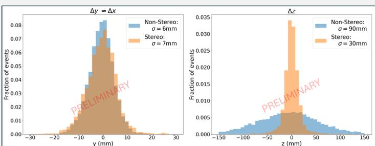
**Fig. 4:** The histograms compare vertex resolution,  $\sigma \equiv$  MSE, for non-stereo (blue) and stereo (orange) setups using conservative estimates when simulating detector performance. The left shows xy-plane resolution, and the right shows z-axis resolution.
