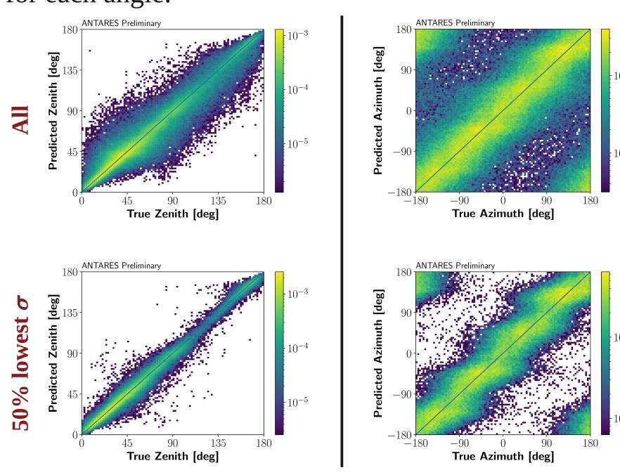
Evaluation of the technique shows an improvement for the zenithal angle compared to the traditional method, as the mean angular error is reduced from 15.5° to 7.5°. Furthermore, in the azimuthal move from total angle we ignorance to a mean error of ~40°, which is considered as a success due to the physical limitation of not having valuable information from other detector lines, while a single line has 120° resolution.
