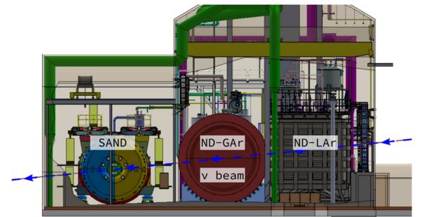
Figure 3: Representation of the ND hall in Phase II, showing its different subcomponents [2].
