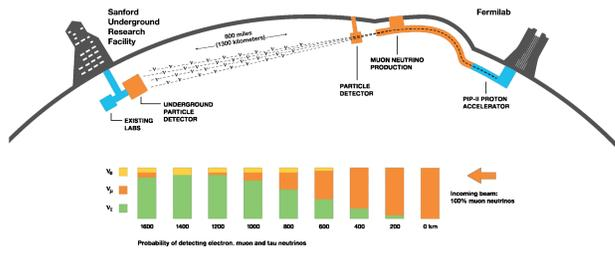
Figure 1: Schematic of the DUNE experiment [1].
