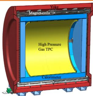
Figure 4: Cross section of the ND-GAr geometry, showing the HPgTPC, ECal and magnet.
