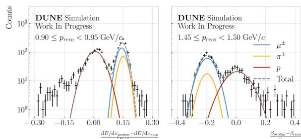
Figure 8: Distribution of  $dE/dx$  measured with the TPC (left) and  $\beta$  measured by time-of-flight with the ECal (right) for two different momentum bins.
