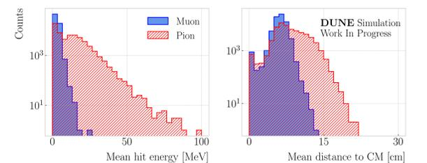
Figure 6: Feature distributions for muons and pions in the range  $0.8 \leq p < 1.5$  GeV/c used for the BDT training.
