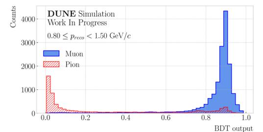
Figure 7: Predicted probabilities assigned by the BDT to true muons (blue) and charged pions (red).
