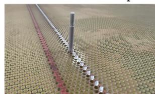
3.2 mm thick rectangular panels glued on the border. Long and delicate procedure with risks due to strip connectivity (soldered) and PCB rigidity.
