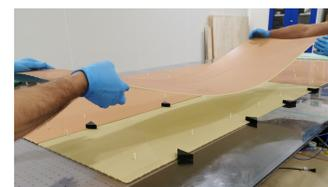
1.6 mm thick panels shaped along strip directions with adhesive tape on one face. Faster and simpler procedure but stringent constraint on hole alignment.
