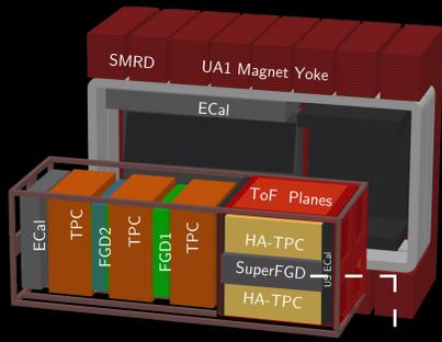
Fig. 1: Schematic of T2K's Upgraded Near Detector ND280.
