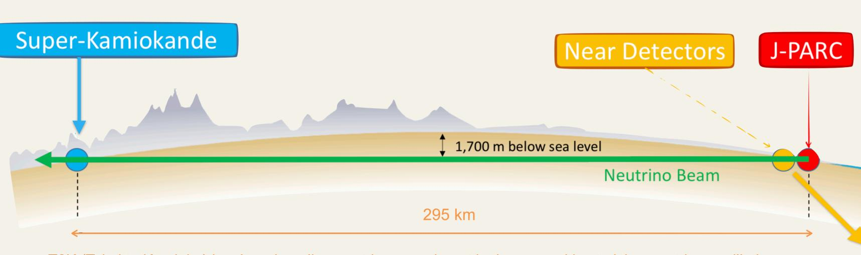
T2K (Tokai to Kamioka) is a long-baseline neutrino experiment in Japan, and is studying neutrino oscillations. Near detector ND280 constrains the neutrino flux and neutrino interaction cross sections for oscillation analysis.
