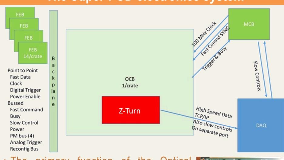
The primary function of the Optical Concentrator Board (OCB) is to move and organise digital data and commands.
