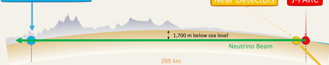
T2K (Tokai to Kamioka) is a long-baseline neutrino experiment in Japan, and is studying neutrino oscillations. Near detector ND280 constrains the neutrino flux and neutrino interaction cross sections for oscillation analysis. Near Detector ND280 upgrade: better constrain  $\nu$ -nucleus interactions and hence improve systematic uncertainties. => Installation completed in May 2024
