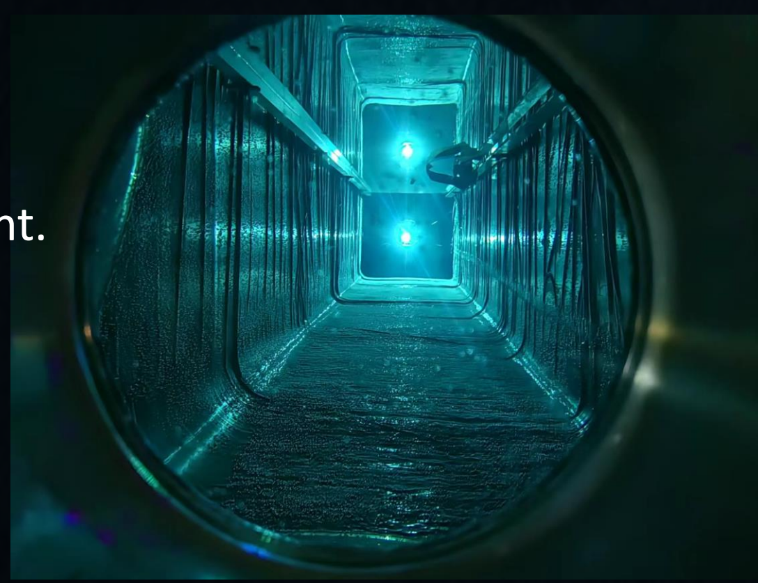
View of LED at the end of the 10m long hDOM and calibration water tank
