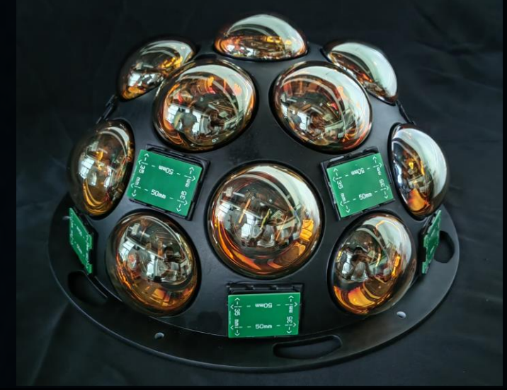
Hemisphere of hDOM prototype with PMTs and SiPM back-end locations
