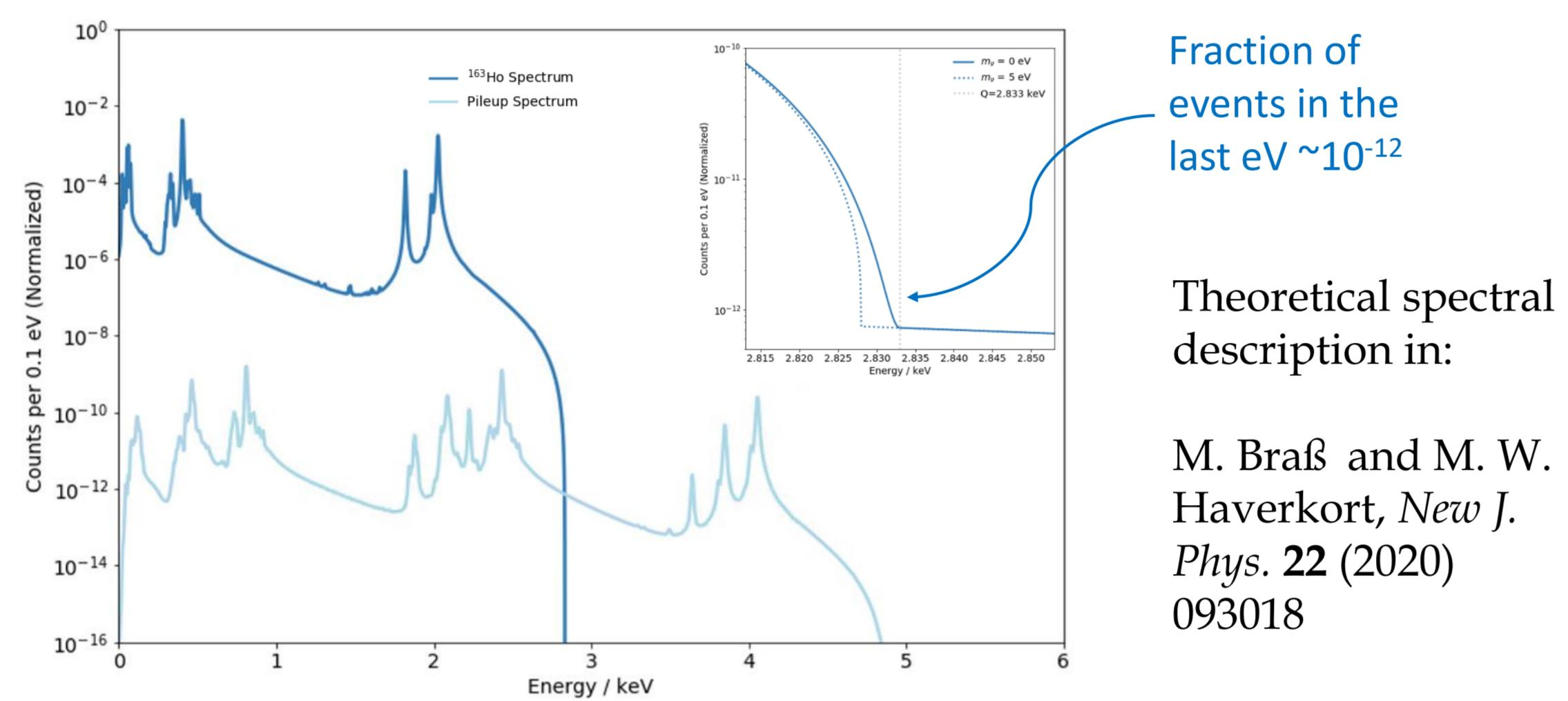
ECHO will perform high energy resolution and high statistics calorimetric measurements of  $^{163}\text{Ho}$  spectra by enclosing  $^{163}\text{Ho}$  in metallic magnetic calorimeters
