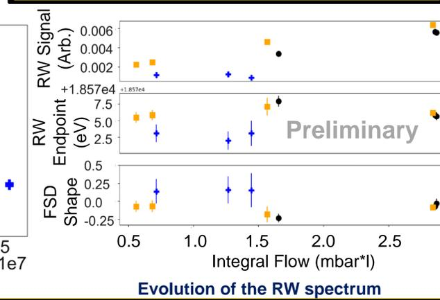
❖ RW spectrum measurements are performed by varying the retarding energy threshold to scan the RW  $\beta^-$  spectrum and then fitting a model to that RW  $\beta^-$  spectrum.
