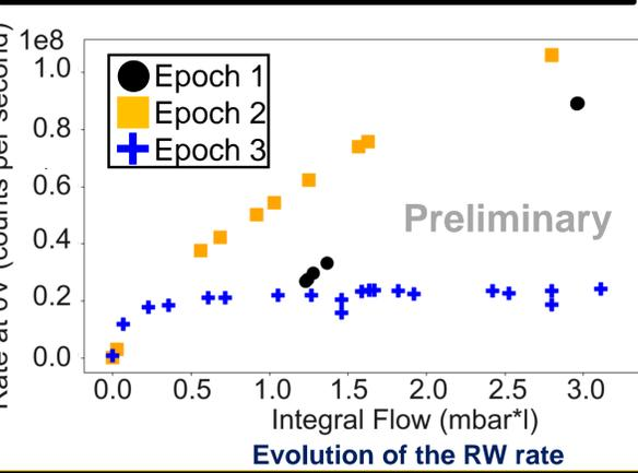
❖ RW rate measurements are performed whenever there is no tritium in the gaseous source (e.g., between KATRIN Neutrino Mass Campaign "KNM" etc).
