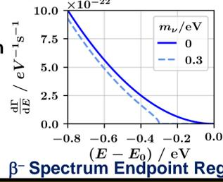
The spectral shape near the endpoint is analyzed to determine the neutrino mass signature.
