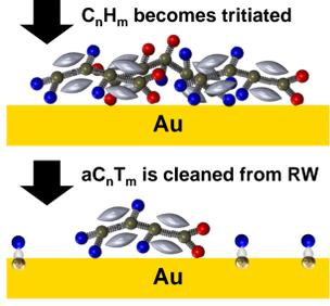
3. The  $aC_nT_m$  has been almost removed. We see that there is limited accumulation of tritium activity (T adsorbs poorly on Au).
