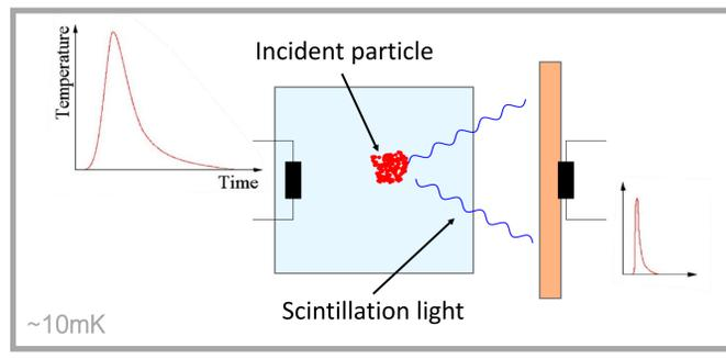
Cryogenic calorimeter used as light detector  $\rightarrow$  Particle identification with light pulse shape
