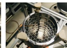
Inside view of the purity monitor field cage. The fiber is inserted in the photocathode grid ring. In the picture the fiber is pointing upward. The photocathode is installed in the last slot of the PEEK holder, with the gold layer facing down.
