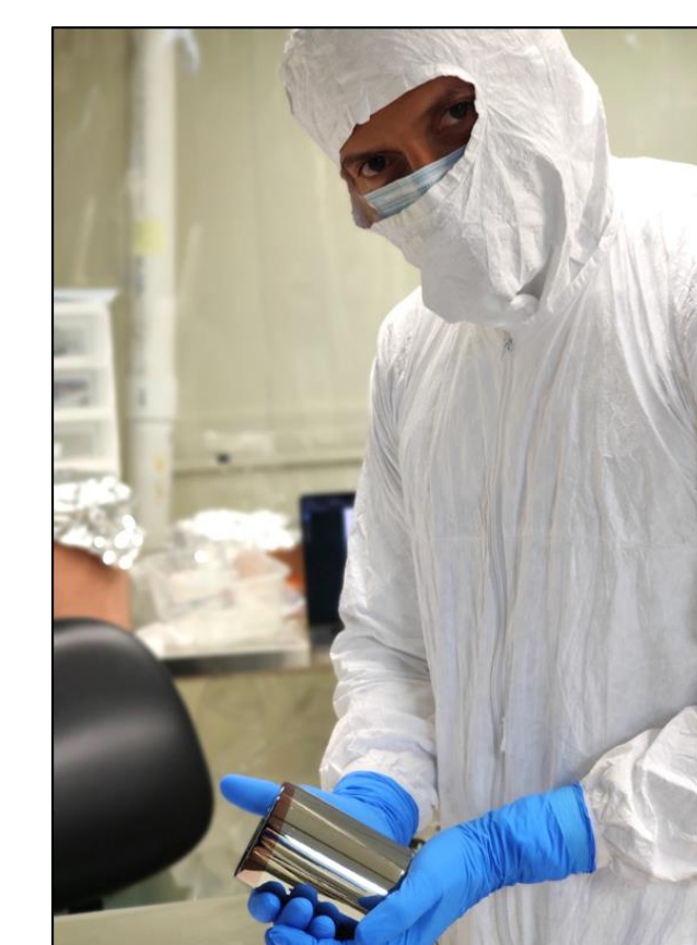
David Hervas holding a recently-decryostated ICPC detector
