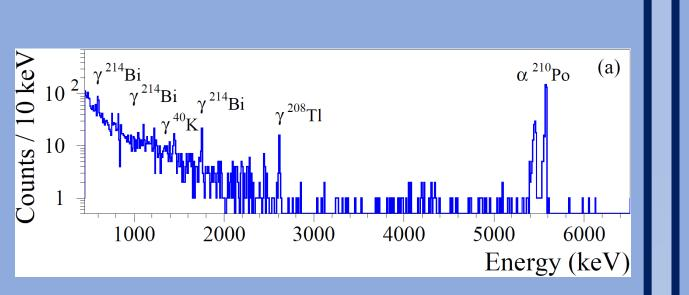
Background spectrum measured by a 0.55 kg <sup>130</sup>TeO<sub>2</sub> bolometer (116 h at 27 mK)
