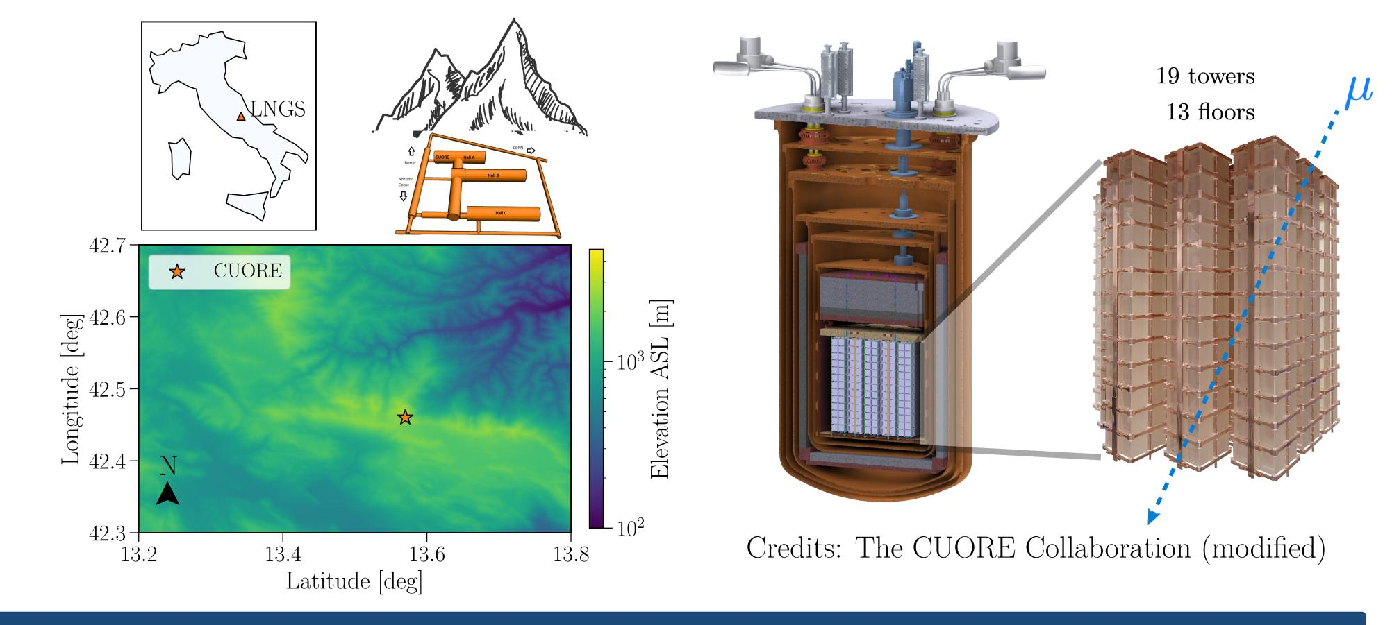
• Detector segmentation into 988 cubic-crystals  $(5 \,\mathrm{cm \ side})$  aids event selection via coincidences. • Segmentation also enables observation of track-like particles such as muons and searches for exotics (see D. Mayer, Contribution #417).
