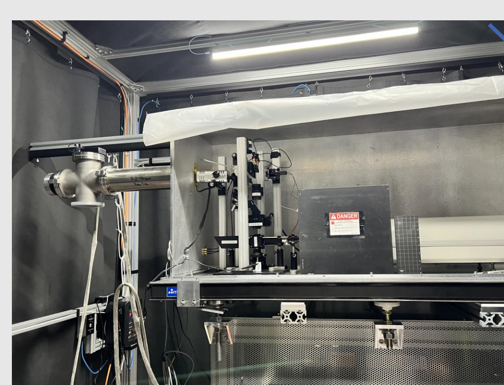
Laser box with optical setup, UV laser, alignment lasers and secondary shutter
