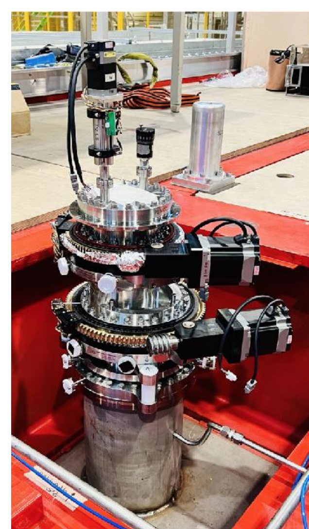
P2: periscope with extra rotation stage
