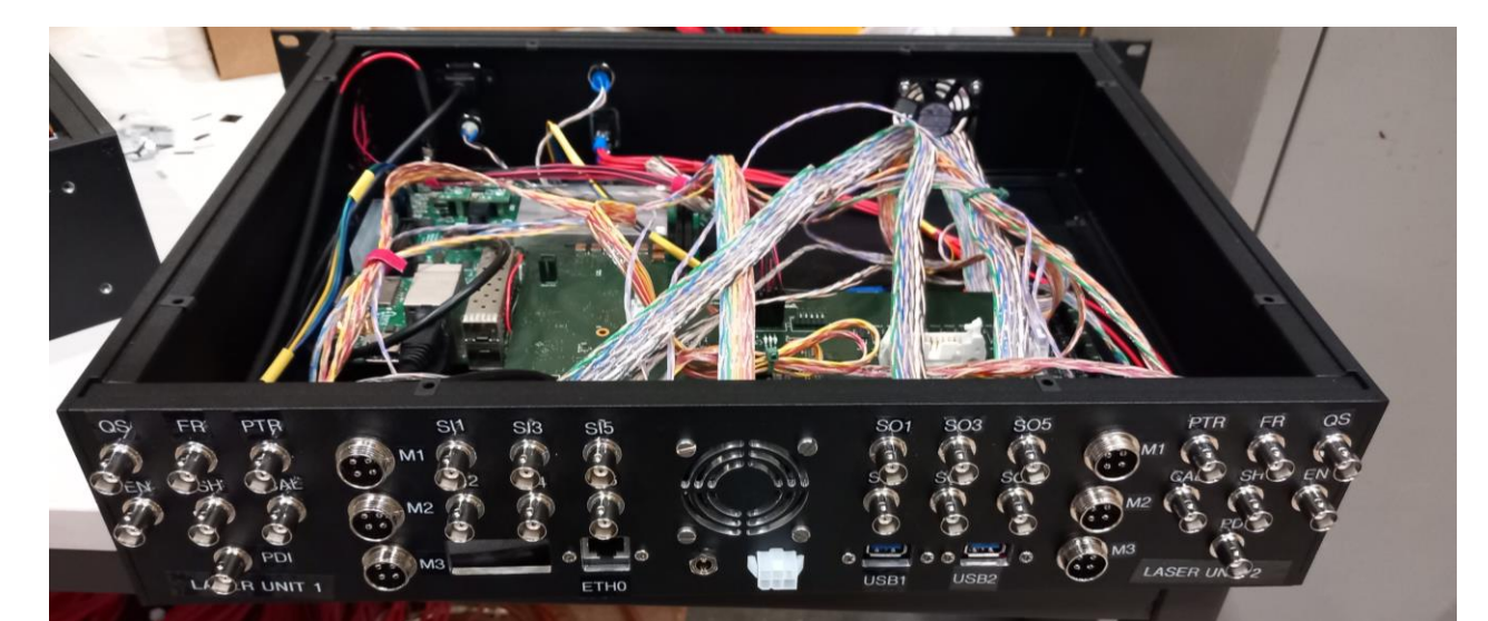
CIB – Calibration Interface Board
