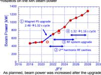
While supplying the beams for the T2K experiment further increase is expected after the RF system upgrade Reaching ~1 MW in 2025 - Reaching 1.3 MW in 2028 (in time for starting Hyper-K operation)
