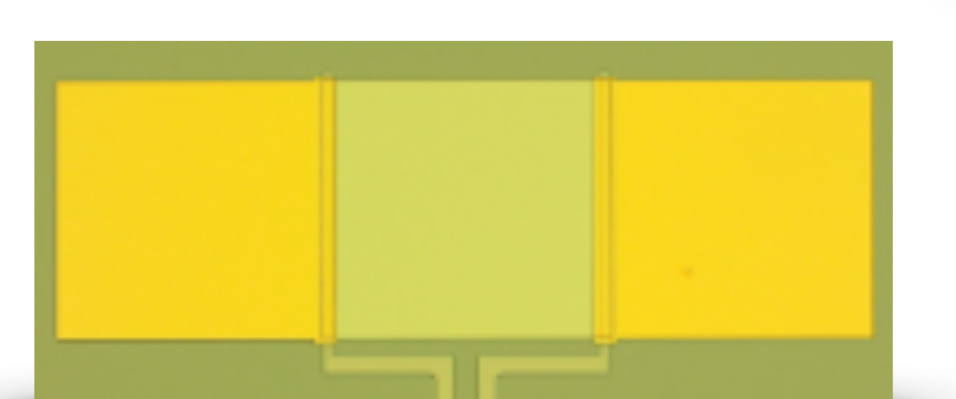
square Ir/Pt bilayer TES in the middle with Au pads on both sides
