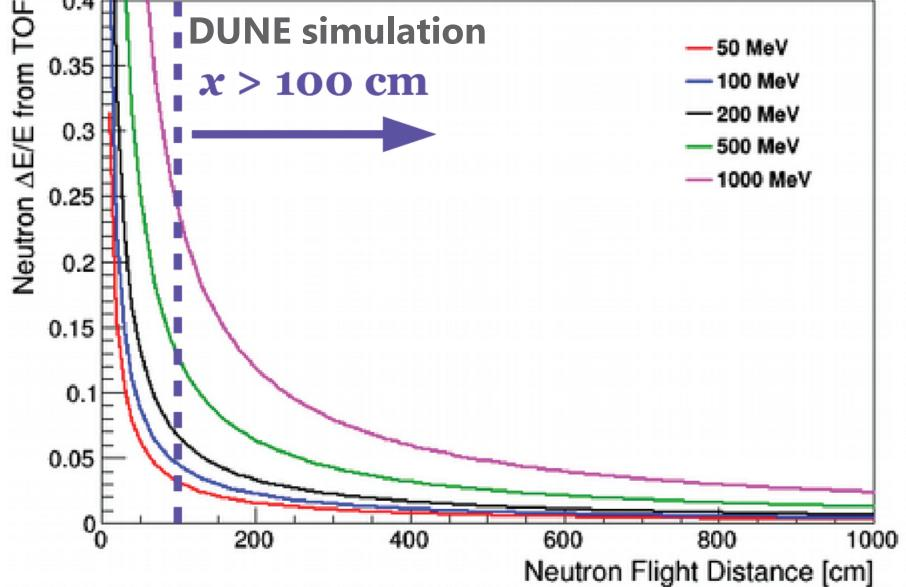
$$v_n = \frac{d(v, p)}{t_p - t_v} \qquad E_n = \gamma m c^2$$
