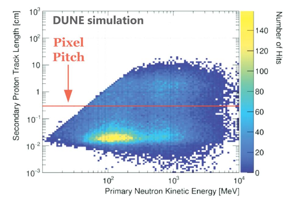
Proton tracks produced by neutrons are usually short [4] and difficult to identify. Need dedicated proton reconstruction software, good time and spatial resolution, and background mitigation.
