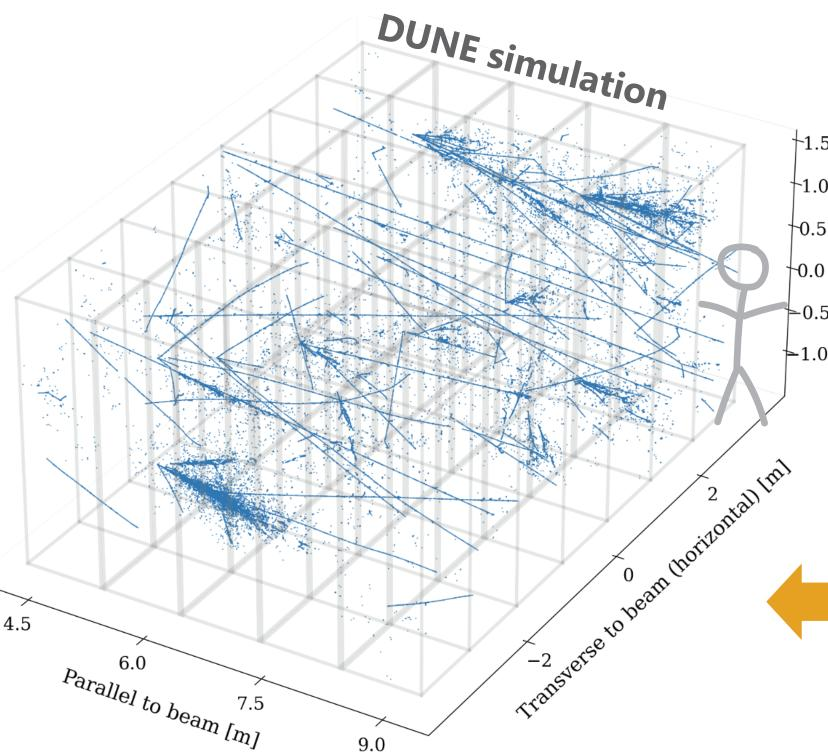
Expect ~50 beam-related interactions per spill in ND-LAr. Extremely hard to find invisible neutrons. Optical segmentation of the detector into 70 TPCs reduces pileup to ~5 interactions per beam spill per TPC.
