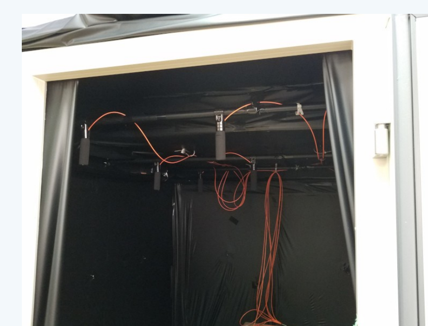
Fiber system for light injection
