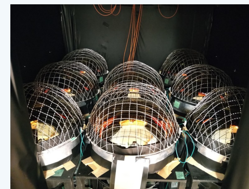
8 PMTs in a room for measurements
