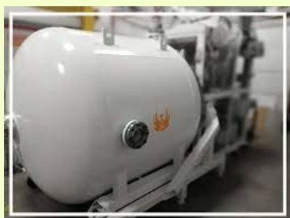
Phoenix – high flux neutron generator [1].
