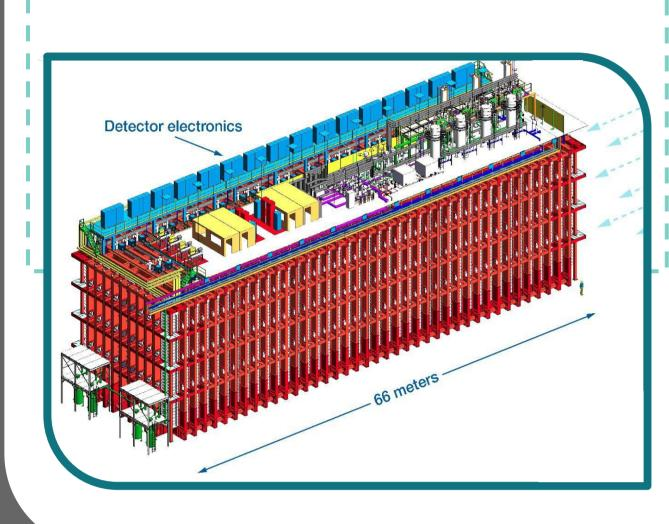
DUNE Far Detector (FD) modules [1]: • Excavation ready to host 4 detectors. •  $17 \text{ kT LAr} \sim 66 \times 19 \times 18 \text{ m}^3 \text{ cryostat.}$
