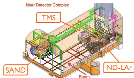
SAND will stand at a fixed position along the beam axis, while ND-LAr and TMS will be movable off-axis, for data-taking in different energy intervals.
