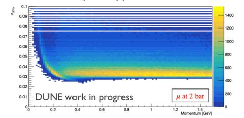
Measured prototype dE/dx resolution
