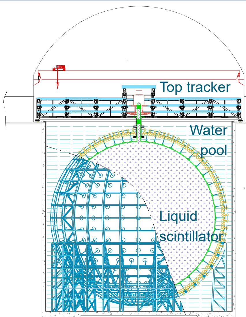
JUNO is multi-purpose liquid scintillator detector under construction in China [1]
