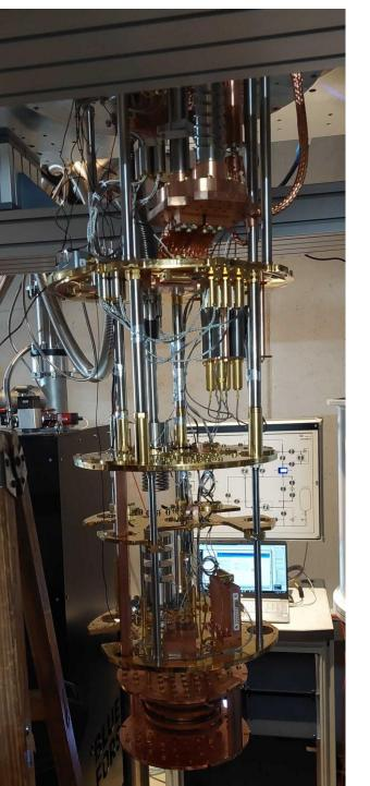
"Dry" Dilution refrigerator to avoid handling of cryogenic liquids. The base temperature reached is below 7mK.
