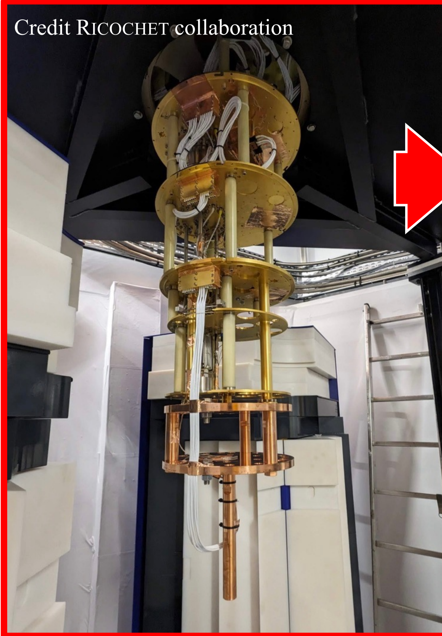
The RICOCHET cryostat during the cryogenic run
