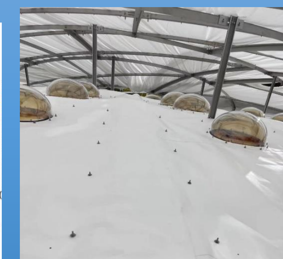
Reflectivity larger than 95% for wavelengths > 300\text{nm}
