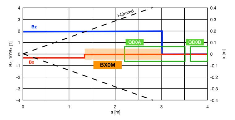
A first corrector **BXOM** is placed just after the beam pipe separation at ±1.285m, to cancel the solenoid Bx.
