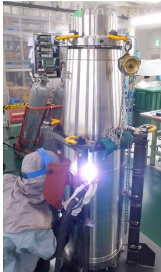
Covering the cold mass with the helium vessel and welding the vessels
