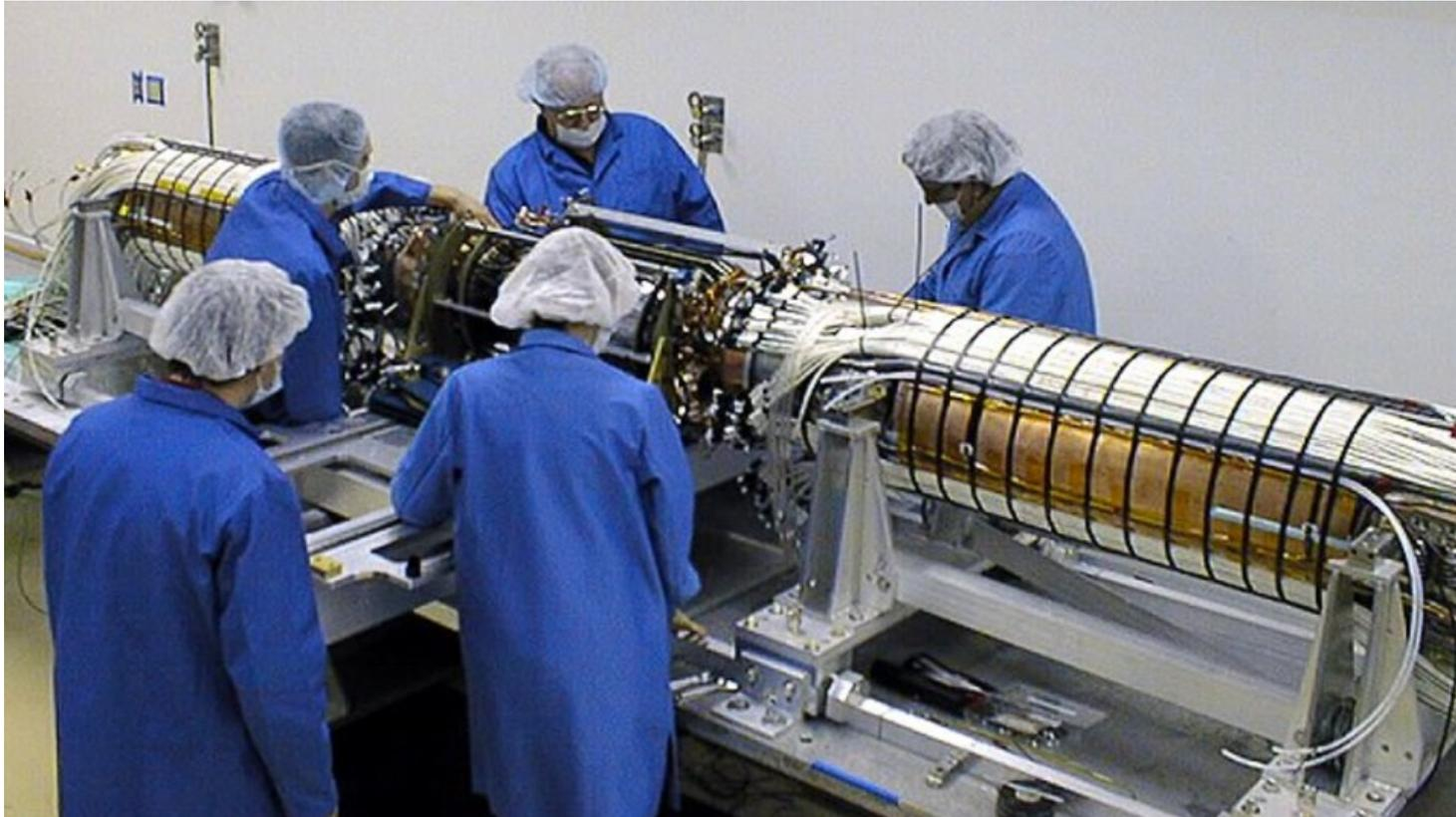
BaBar's vertex chamber mounted on Be chamber. Vertex cables are mounted over the PM IR magnets together with accelerator cables, cooling, and diagnostics.
