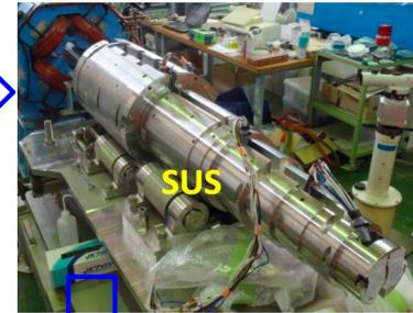
Measurement of quadrupole alignment in the cold mass with the stationary harmonic coil at room temperature
