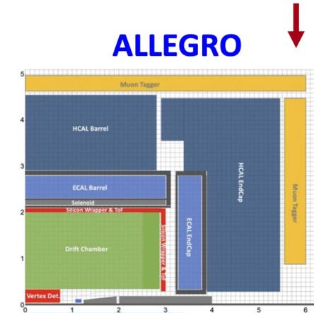
Radial removal of detector end chambers is much easier. In and out in ~day. Longitudinal end chamber removal will take ~weeks with poor vacuum for perhaps another week.
