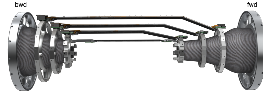
Combined Support Cooling Block (SCB), manufactured using 3D printing technology, with CO 2 and N 2 channels inside.
