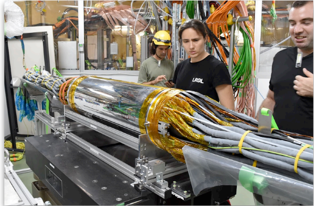
VXD ready for installation into Belle II
