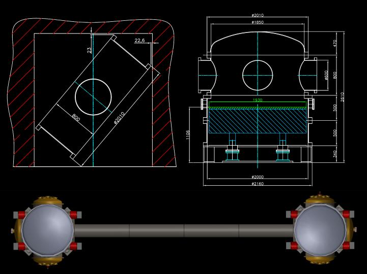
Two chambers connected by vacuum pipe.
