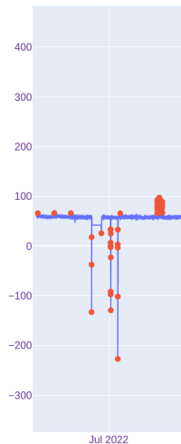
Figure 16: Anomalies detected by the IQR method on the ups sensor value [kW].
