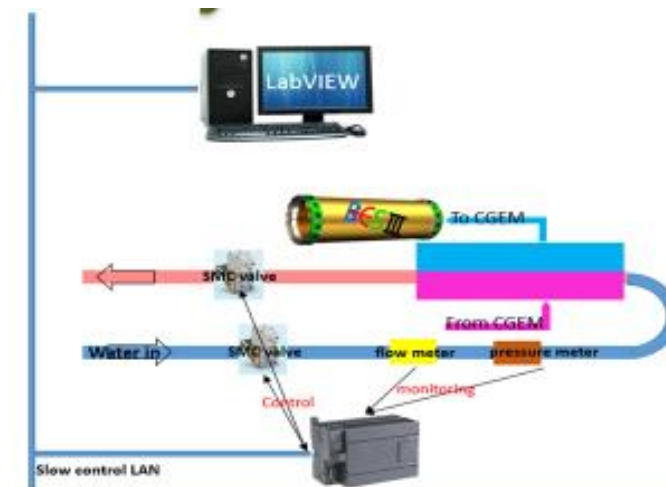
Cooling control and monitoring architecture (PLC option)
