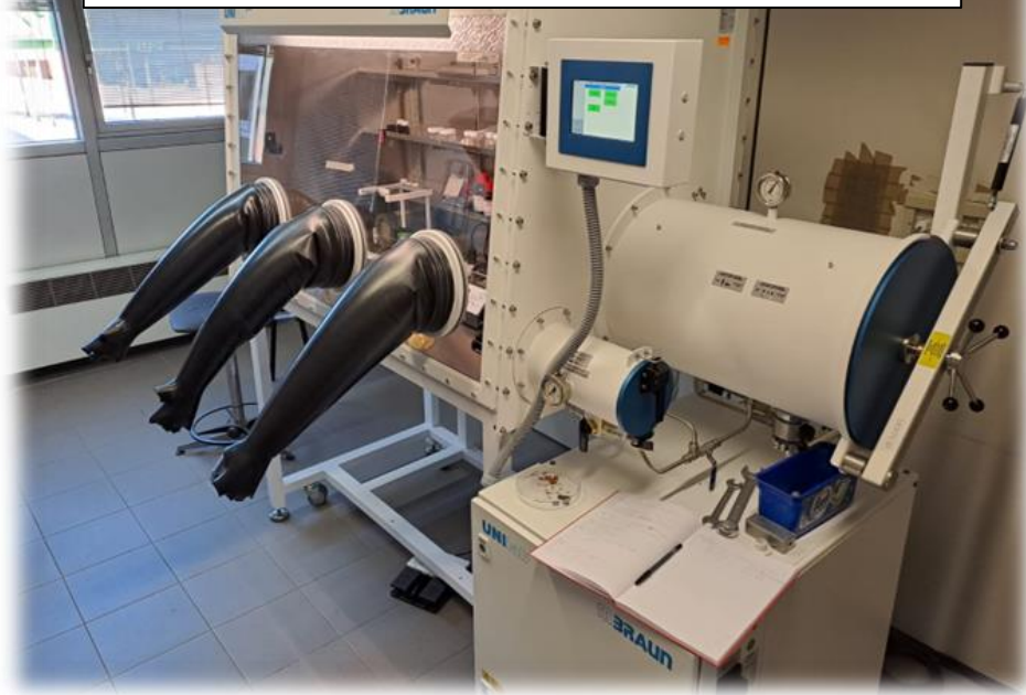
Equipped glovebox: spin coater, hot plates, microbalance
