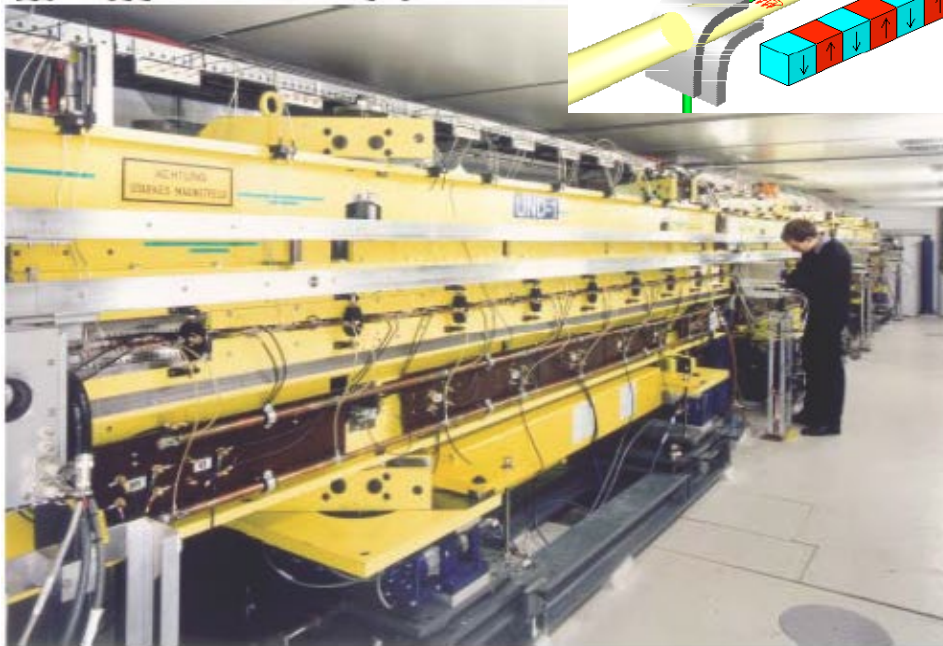
Fig. 1.3 Left: Magnetic undulator for the X-ray laser XFEL [179]. The picture is taken from [180]. Right top: laser-ablated diamond crystal. The crystal size is 4 \times 2 \times 0.3 \text{ mm}^3 . The undulator period is \lambda_u = 50 \mu\text{m} . The picture is taken from [74]. Right bottom: a \text{Si}_{1-x}\text{Ge}_x superlattice crystalline undulator with four periods. Periodically varied Ge content (from x = 0 to x_{\text{max}} = 0.5\% ) gives rise to the undulator period \lambda_u = 50 \mu\text{m} . The picture is courtesy of J.L. Hansen, A. Nylandsted and U. Uggerhøj (University of Aarhus).
