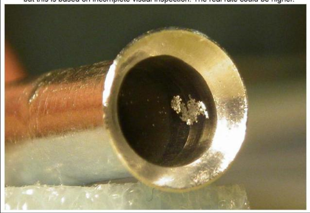
We have discovered corrosion in this short pipes that connect the detctor to the cooling system.
