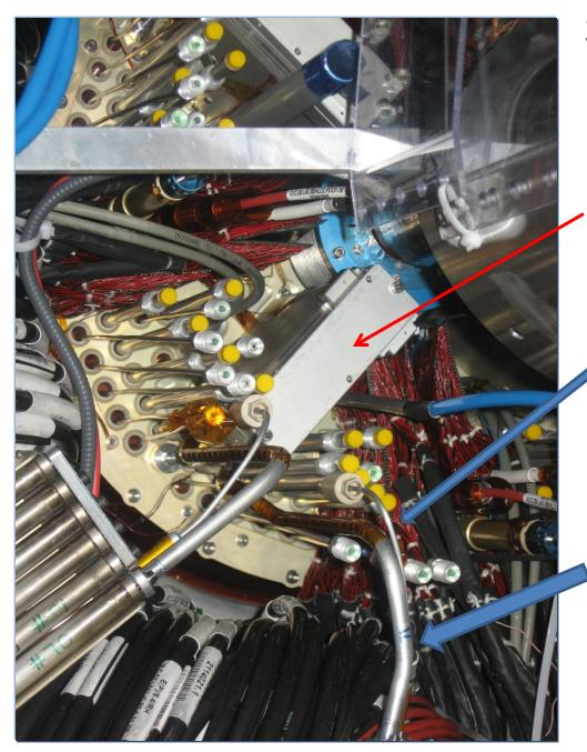
Zoom in of the pp1 connection location for fibers and cooling pipes.
