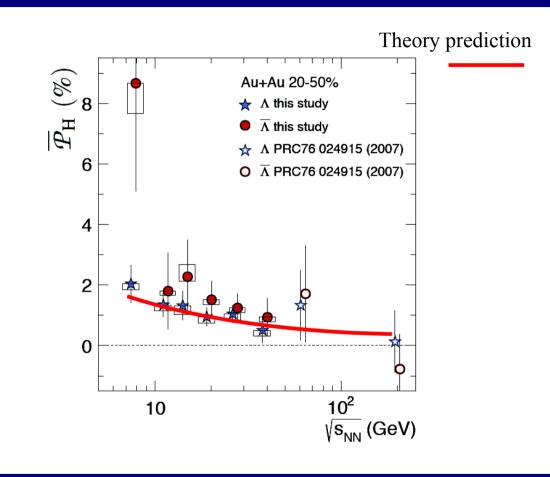
Particle and antiparticle have the same polarization sign. This shows that the phenomenon cannot be driven by a mean field (such as EM) whose coupling is *C-odd*. In agreement with the predictions based on spin-vorticity formula
