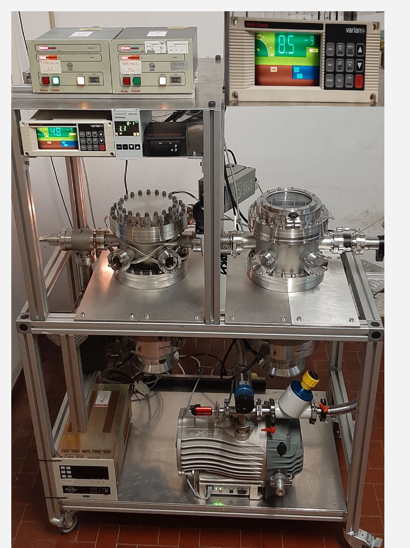
Experimental Setup for outgassing studies @ University of Bari and INFN
