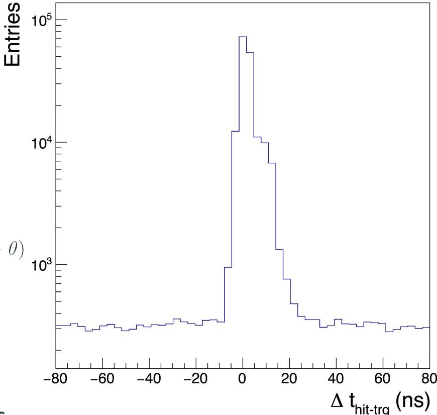
Using the timing scintillators downstream our detector we can select signal hits in time with the incoming beam particle
