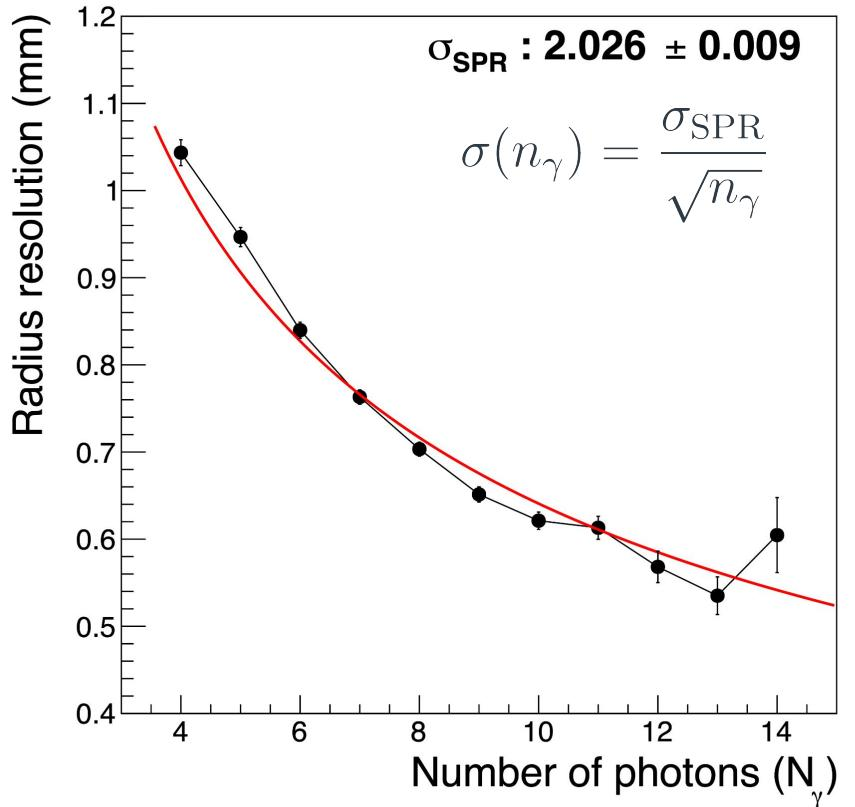
We can calculate the single-photon resolution by fitting this curve
