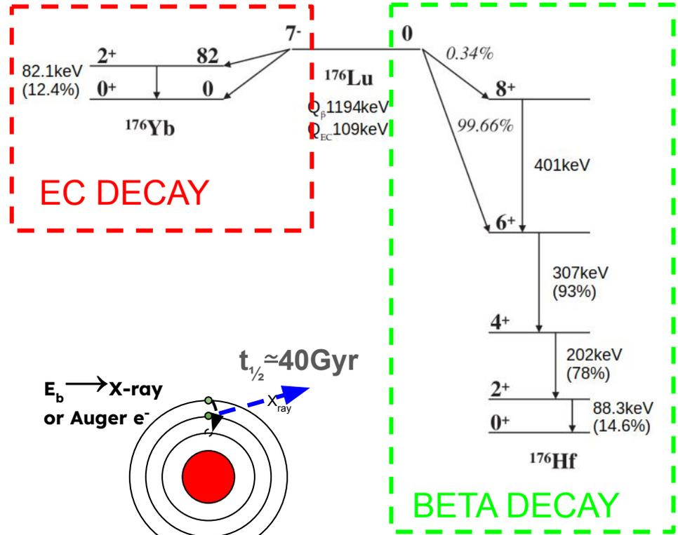
Previous searches for the  $^{176}\text{Lu}$  EC decay were performed by using a passive Lutetium source coupled to a HP-Ge detector.
