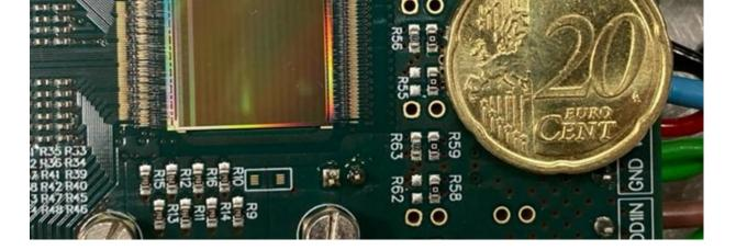
Pixel pitch 25 µm Power consumption  $O(10 \text{ mW/cm}^2)$ Digital Readout
