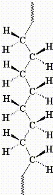
The formation of a branched structure has dramatic consequences on the physical properties of the so produced polyethylene. In the case of branched structure only LOW DENSITY POLYETHYLENE will be obtained (LDPE). The structure not only affects the density but also the **degree of crystallinity**, which in turn affects several important technological properties of the product, as we will see... Linear PE can be obtained ONLY through **Ziegler-Natta polymerization....**
